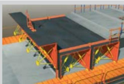
For the second pour, four of the half tunnels are moved to the next position. One half tunnel remains in place as it is supporting a section of slab on the first pour. On the second phase, two walls and two slabs are poured, creating a further four bedrooms.
