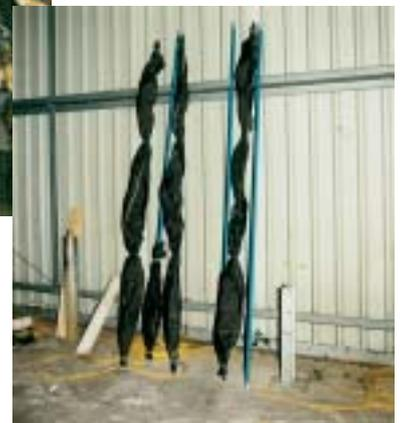
inserted into the cased hole and a grout mix is injected through the hollow bar at 8-12 bar pressure to fill the sock. The pressure forces the water from the grout mix out of the geotextile's fine mesh, leaving the cement to cure almost instantly within the sock.
